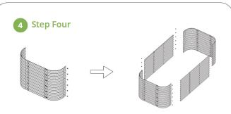
After straight panels are assembled, attach corner panels with straight panels using the same method. Make sure corner panels are attached outside of the straight panels. (Please refer to Bracing Rod Installation Guide for rod assembly instruction.)
