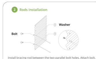
panel, washer & rod loosely, making sure that the rods are connected to the **third** and **fifth** bolt holes from the top. Then tighten them up by screwdriver for reinforcement of raised bed.
