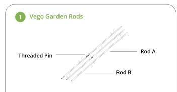
Vego Garden bracing rods are used to reinforce the strength of oversized raised beds. For 2.5ft wide raised bed: use Rod A only; For 4ft wide raised bed: use the Threaded Pin to assemble Rod A & Rod B.
